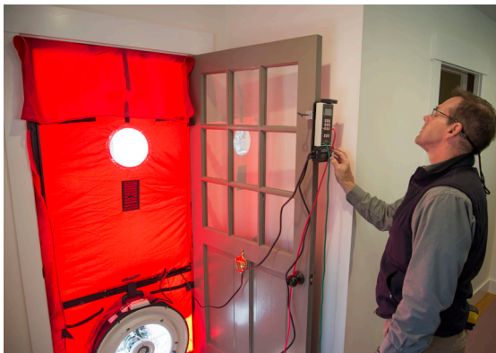
A blower door test was conducted before and after renovations to create negative air pressure and highlight areas of air leakage.
