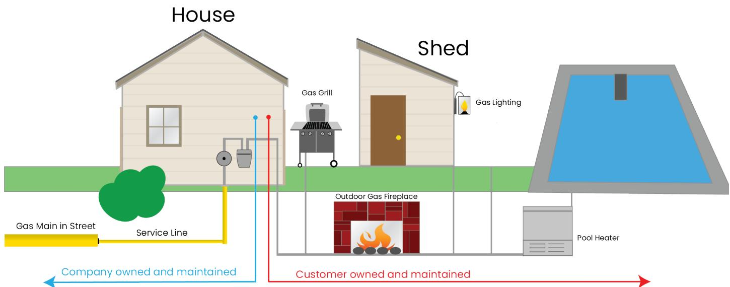
These examples are not all-inclusive. You must make your own determination of whether you have buried piping extending beyond your meter. To properly care for a buried pipe, it is recommended that the pipe be inspected periodically for leaks and corrosion if lines are metallic.
