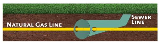
A blocked sewer line may be the result of another utility line (gas, electric, telecommunications) accidentally cross boring through the sewer line. A cross bore is an unsafe intersection of two different utility lines. Do not try to clear a sewer line blockage yourself. It could result in a serious accident. The safest way to ensure there is no cross boring in your sewer line is to have a professional inspect the line with a video inspection system.
