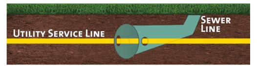
A blocked sewer line may be the result of another utility line (gas, electric, telecommunications) accidentally cross boring through the sewer line. A cross bore is an unsafe intersection of two different utility lines. Do not try to clear a sewer line blockage yourself. It could result in a serious accident. The safest way to ensure there is no cross boring in your sewer line is to have a professional inspect the line with a video inspection system.
